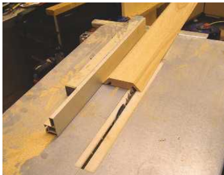
▲ Pic.7 Cut the grooves in the rear post for the infill panels using the table saw with the blade at 45°. The guard has been removed for clarity
